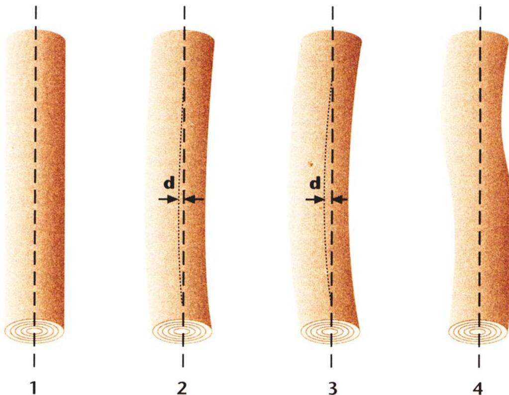
**Figure 1:** Logs 1 and 2 qualify as straight logs; logs 3 and 4 are not straight. Maximum deviation ( $d$ ) on log 2 does not exceed 1 cm over 1 m length. Maximum deviation ( $d$ ) on log 3 exceeds 1 cm over 1 m length. Log 4 shows bow in more than one direction.
